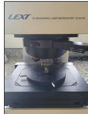
Figure 3. Experimental inspection of roughness using the laser confocal.
